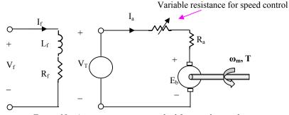
Figure 18: Armature resistance method for speed control
