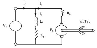
Figure 9: Shunt DC Motor
