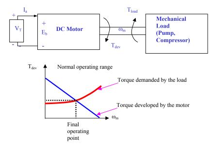
Figure 12: Interaction of the DC Motor and Mechanical Load
