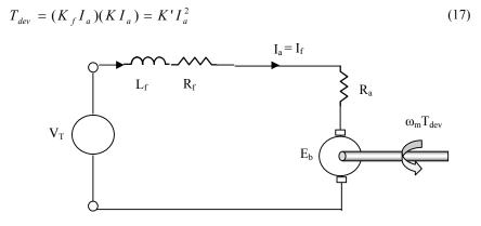
Figure 10 (redrawn): DC Series motor equivalent circuit
