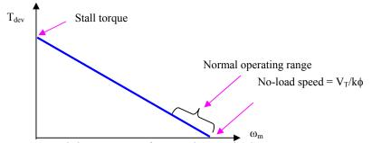
Figure 11: Torque-speed characteristics of separately excited DC motor
