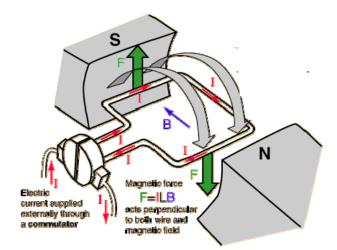
Figure 4: Torque production in a DC motor
