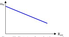
Figure 19: Variation of speed with external armature resistance
