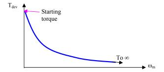
Figure 13: Torque-speed characteristics of a series motor
