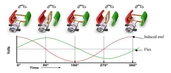
Figure 5: Induced voltage in the armature winding of DC motor
