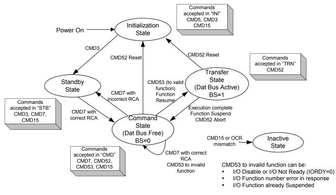
Figure 6-2 State Diagram for Bus State Machine
