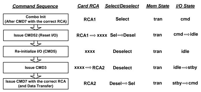
Figure 3-8 Re-Initialization Flow for I/O Controller
