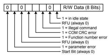
Figure 5-3 IO\_RW\_DIRECT Response in SPI Mode
