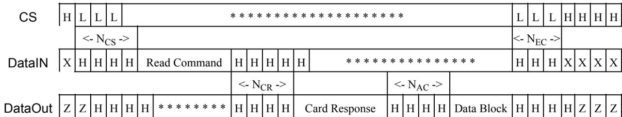
**Figure 53: Read Single Block operations - bus timing**
