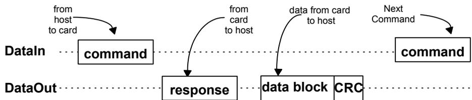
Figure 40: Single Block Read operation
