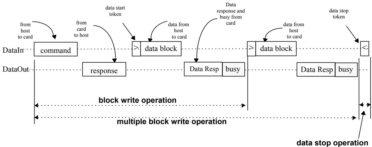
**Figure 13: Write operation**
