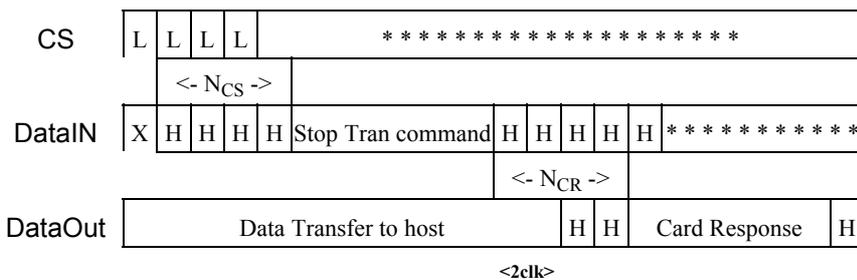
**Figure 54: Stop Transmission in Read Multiple Block**
