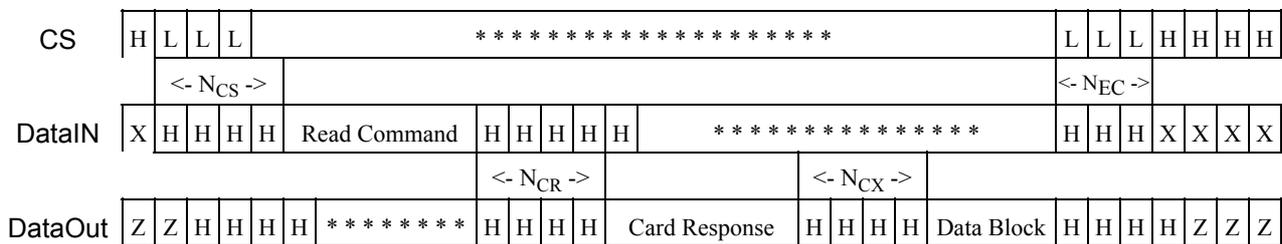
**Figure 55: Read CSD / CID - bus timing**
