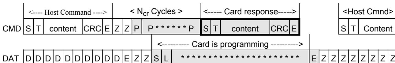
**Figure 33: Stop transmission during data transfer from the host**
