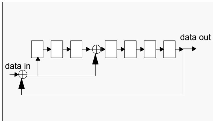
Figure 20: CRC7 generator/checker
