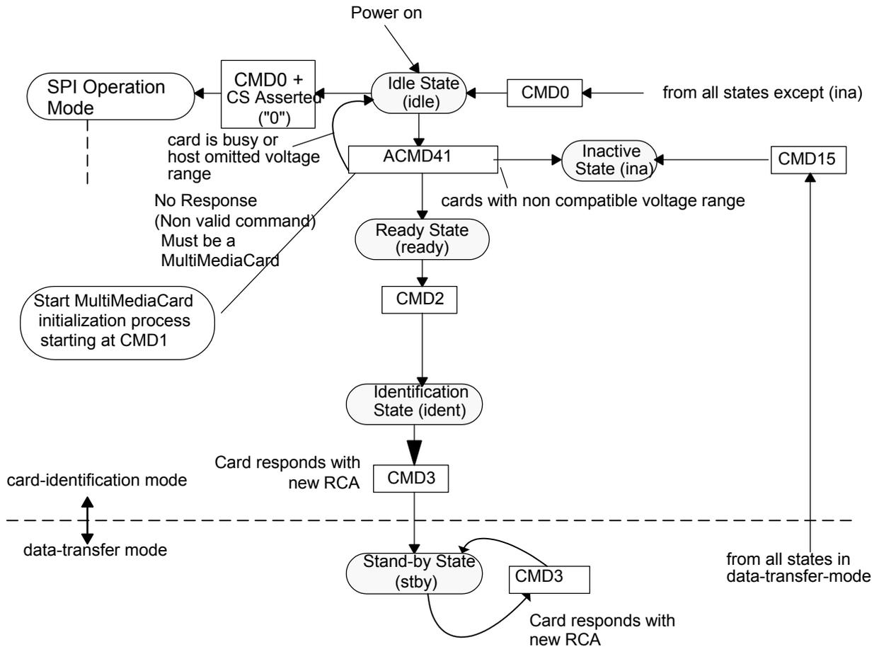
**Figure 14: SD Memory Card state diagram (card identification mode)**
