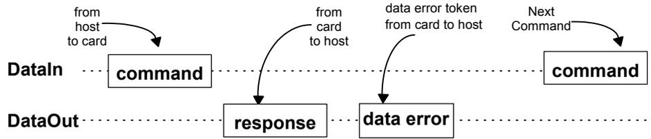
**Figure 41: Read operation - data error**
