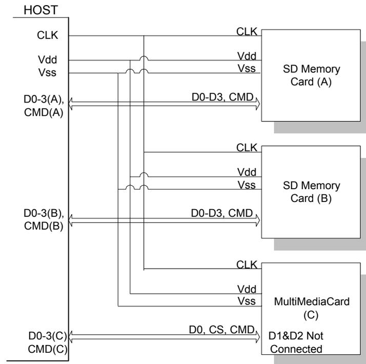
**Figure 2: SD Memory Card system bus Topology**
