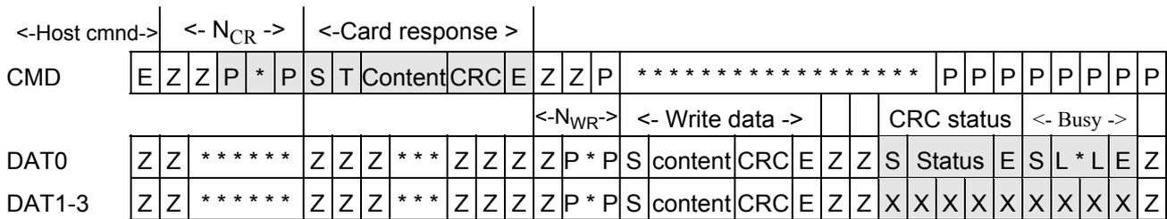
Figure 31: Timing of the block write command
