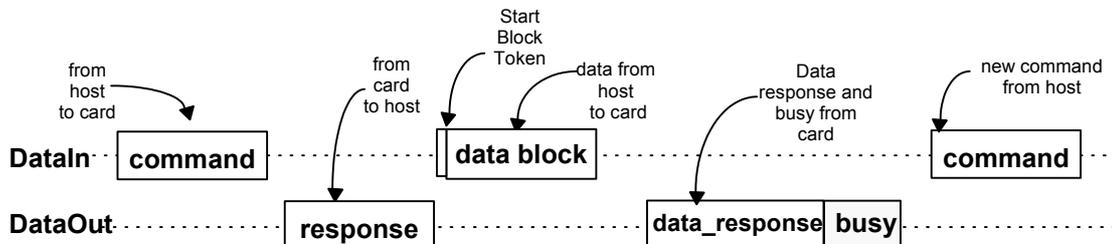
**Figure 43: Single Block Write operation**
