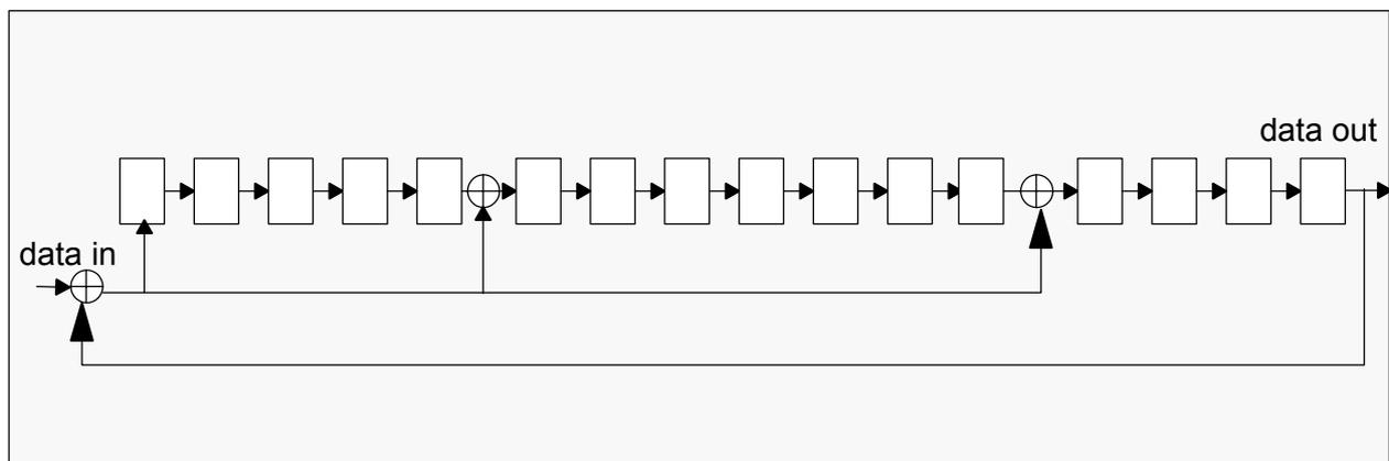
Figure 21: CRC16 generator/checker
