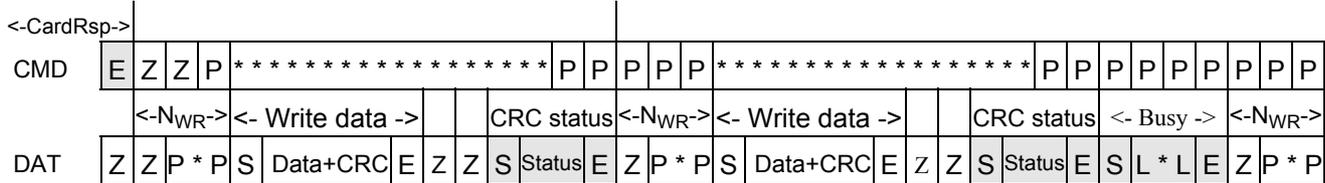
Figure 32: Timing of the multiple block write command
