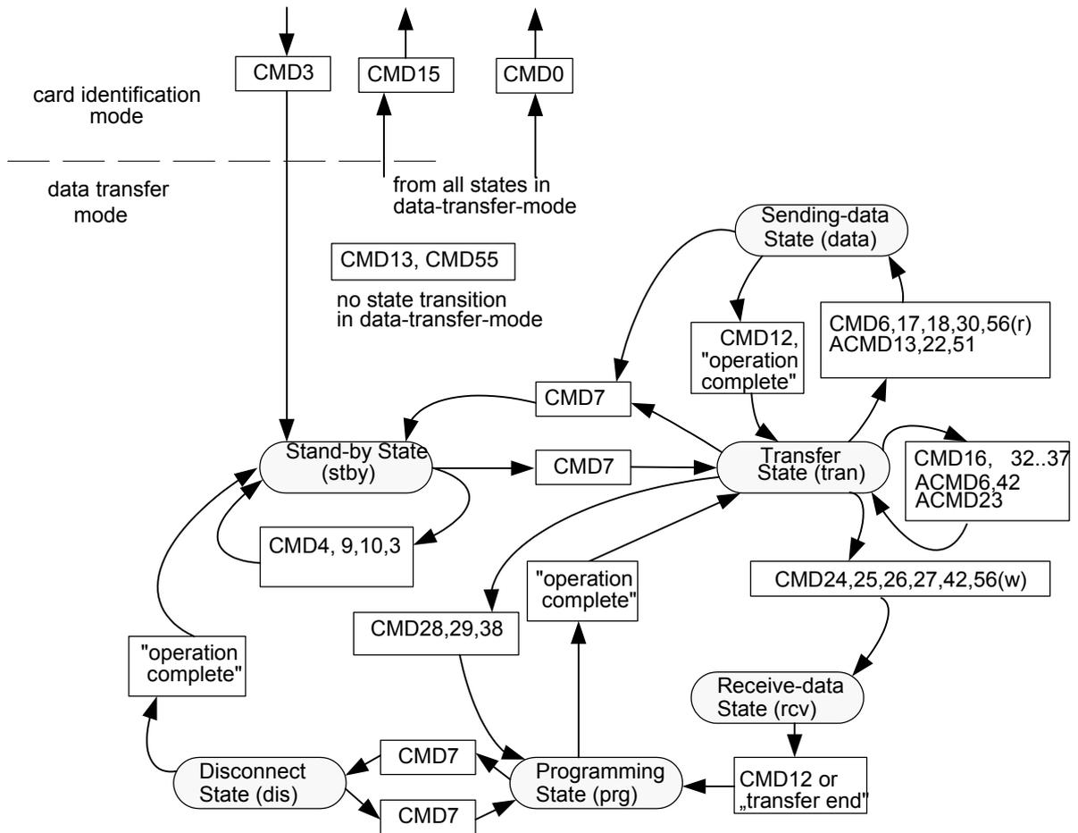
**Figure 15: SD Memory Card state diagram (data transfer mode)**
