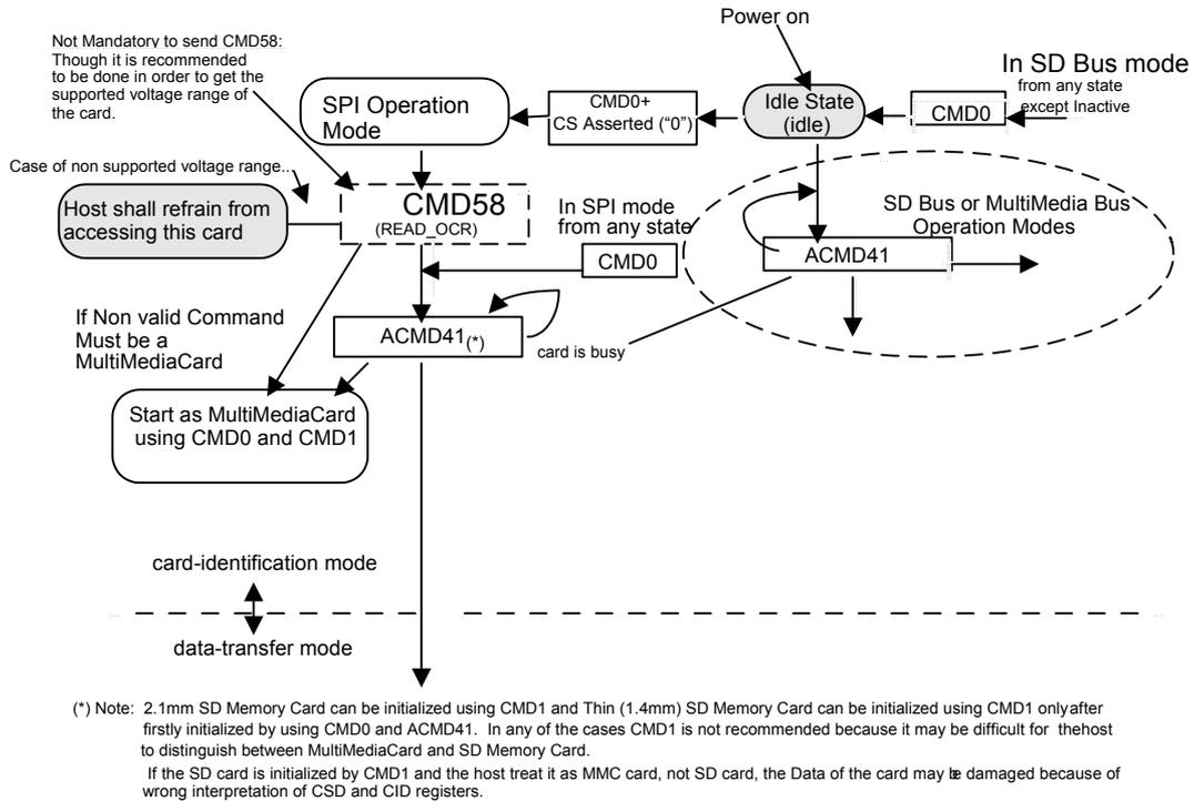
**Figure 39: SPI Mode Initialization Flow**
