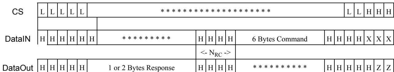
**Figure 52: Timing between card response to new host command**
