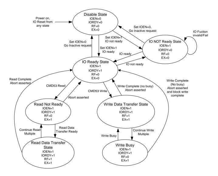
Figure 8 State Diagram for Function State Machine
