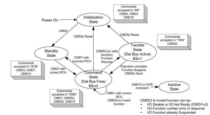
Figure 7 State Diagram for Bus State Machine
