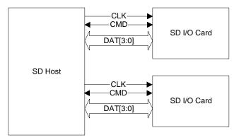
Figure 1 Signal connection to two 4-bit SDIO cards
