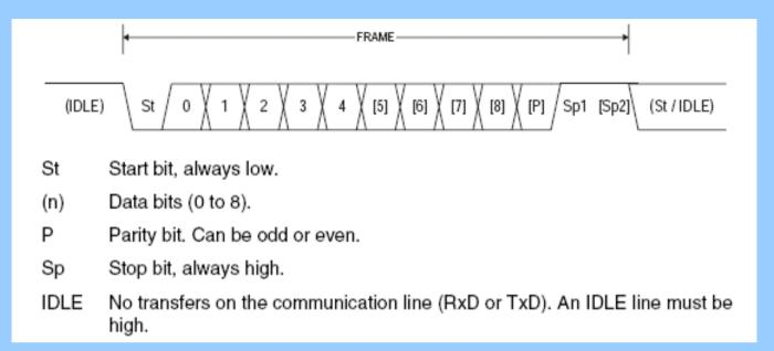
Every frame will have at least -one start bit -some data bits (5,6,7,8 or 9) -one stop bit Parity is optional
