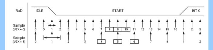
The incoming data is continuously sampled until a falling edge is detected. Once detected, the receiver waits 6 clocks to begin sampling.
